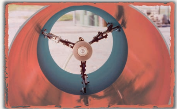
Air-motor controlled adjustable carriage legs quickly center the paint head within the pipe.
