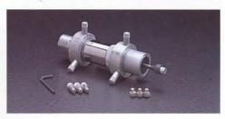
Hollo-Blast is supplied with 1/2" orifice nozzle. However, 5/8" orifice nozzle is also available, where sufficient air supply can be furnished. Air consumption is 200 CFM on 1/2" nozzle; 350 CFM for 5/8" nozzle.
