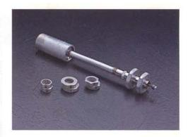
Hollo-Blast Junior is assembled with one standard tungsten carbide nozzle that requires 80 CFM of compressed air. Four sets of centering collars are furnished with the unit to permit adjustment to various sizes within the 1" to 2" range. Tool by itself will slide into 3/4" I.D.
