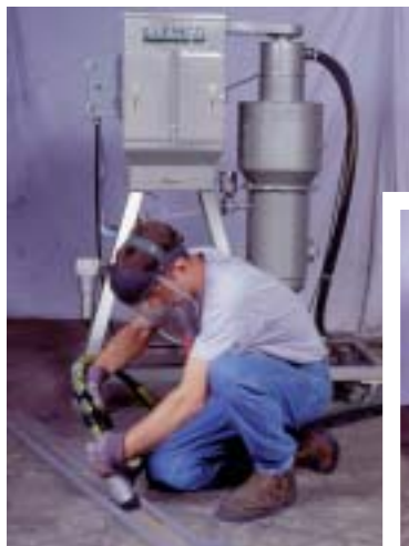
Super Comet with inside angle brush cleans a path 1-inch wide up to 72 inches per minute.
