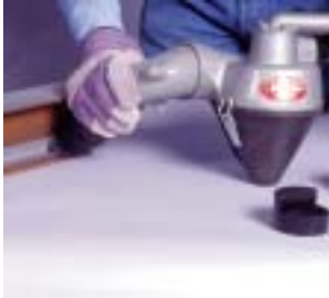
Educt-O-Matic with angle attachment for inside corners.
