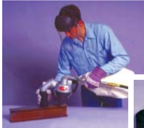
Educt-O-Matic with flat-lip attachment for smooth surfaces.
