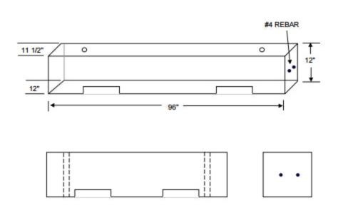
Note: Steel Grade 40 4000 PSI Concrete 5% air entrained
