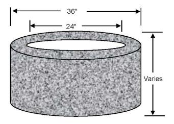
Extensions are available in 6", 12", 18" & 24" heights Extensions are 4000 psi concrete - steel reinforced
