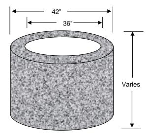
Well rings are available in 12" & 24" heights Well rings are 4000 psi concrete - steel reinforced
