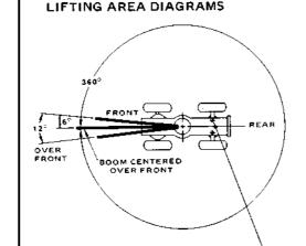
REAR AXLE OSCILLATION LOCKOUTS -MUST BE SET TO MAINTAIN 360
