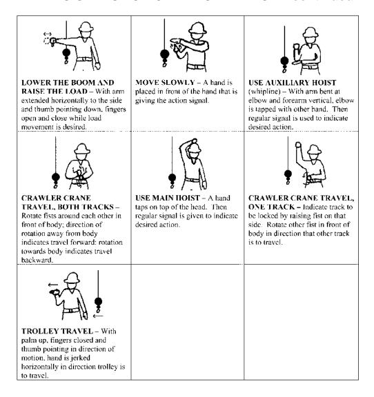
Source for hand signals: OSHA 29 CFR 1926, Subpart CC, Appendix A
