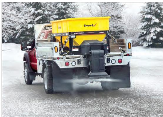
SuperMaxx II spreaders feature an enhanced material feed system with a new stainless steel trough, where brine and salt are mixed before being delivered to the spinner.
